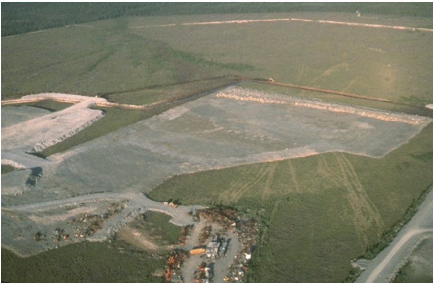
Fig. 9.11 Aerial photograph of an operating zinc mine in Quebec. Iron oxidation is visible as brown stain. The light brown line at the horizon is a ditch that had been dug to intercept the drainage leaving the property of the mine waste management area. (Photograph by Boojum Research)
