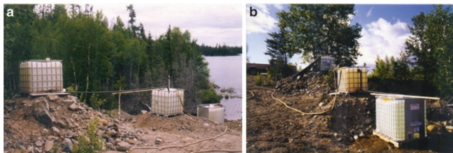
Fig. 7.13 Field pilot test of Mg alloy surfaces in AMD for defining amount of Mg needed to be suspended to buffer decreasing seasonal pH decline. (a) A cascade of three 1 m 3 polyethylene containers. (b) Second experimental setup. (Photographs by Boojum Research)
