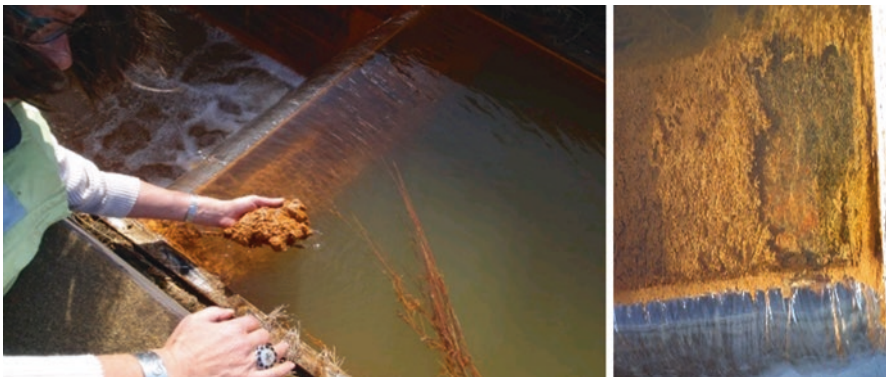
Fig. 9.6 Two photographs of periphyton heavily-caked with oxidized iron at each weir within the pond system and at its edges. (Photograph taken in 2009 by Boojum Research)
