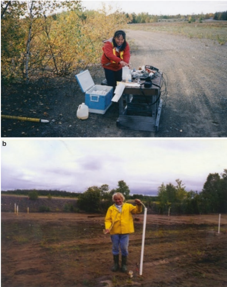
Fig. 6.11 (a) Yan Gan is shown performing the field tests on the activity of a commercial ureolytic enzyme. (b) Murray Johnson shown installing injection standpipes in the sandy area to a depth of 0.5 m which served as the field pilot. A urea-sugar mix was injected about 15 to 20 cm into the sand. (Photographs by Boojum Research)
